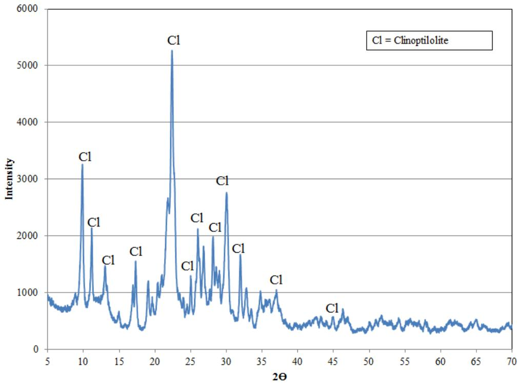
Figure A6: XRD plot of crystalline Zeolite-Z
