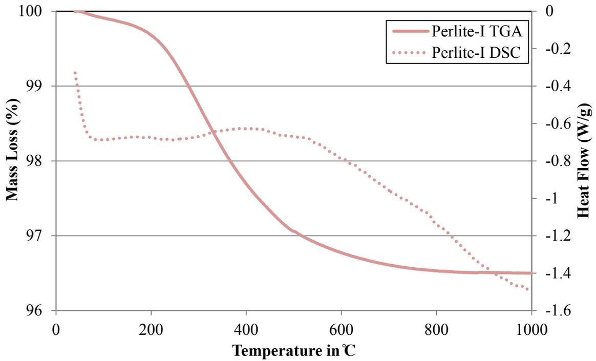
Figure A11: TGA/DSC plot of Perlite-I
