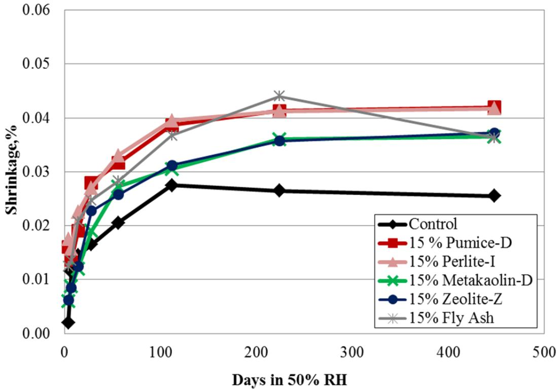
Figure 4.3: Percent shrinkage of concrete mixtures with 15% SCM
