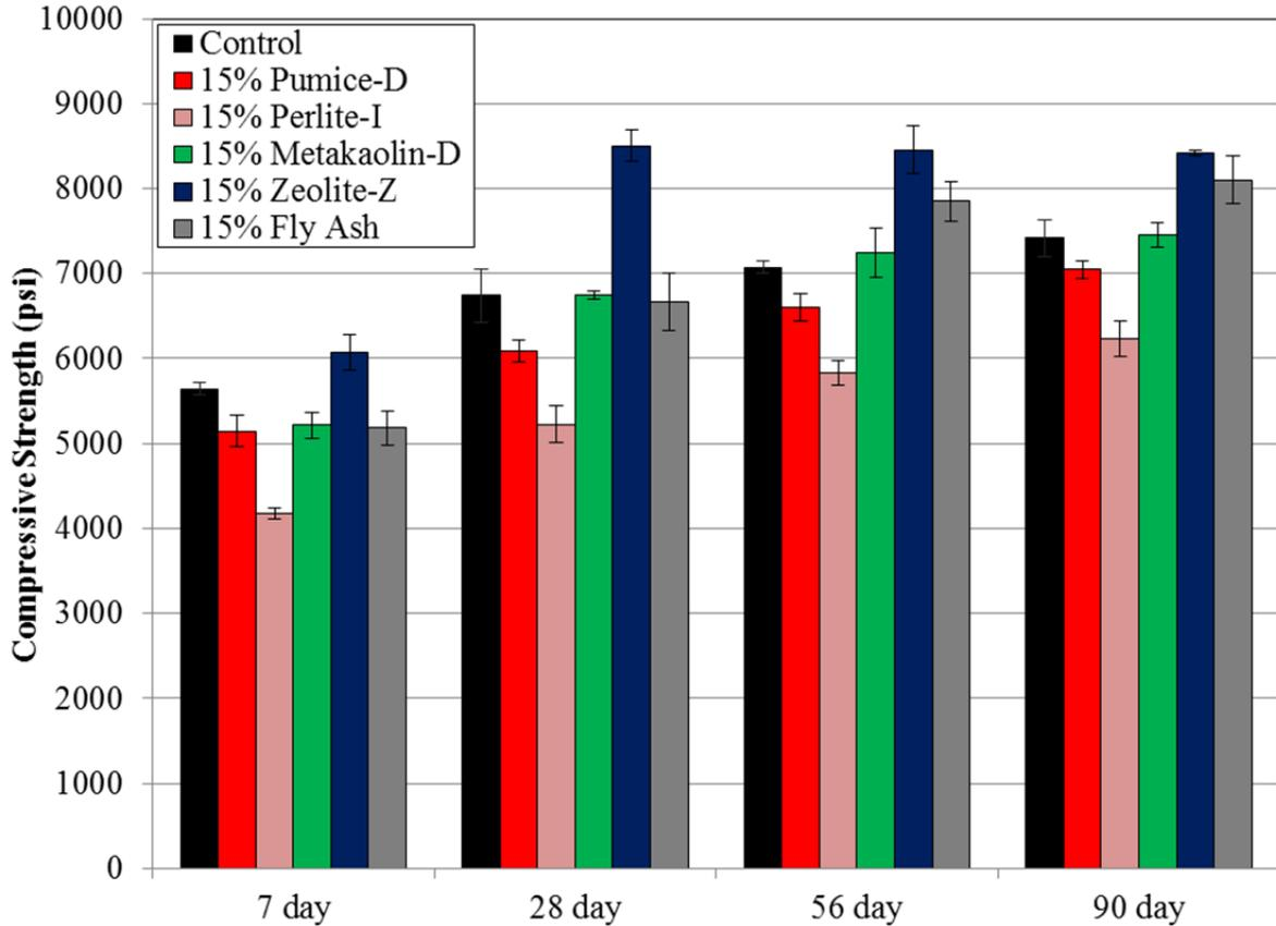
Figure 4.1: Compressive strength of concrete mixtures with 15% SCM
