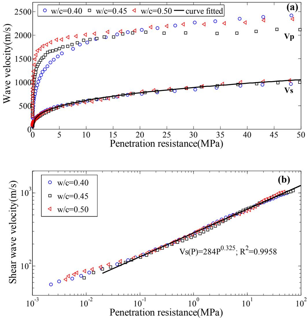
Figure C4: Correlation between  $P$  and shear wave velocities and penetration resistance on mortar mixtures with different  $w/c$  in (a) linear scale and (b) logarithm scale (shear wave velocity only)
