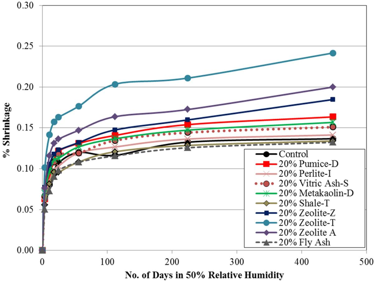
Figure 3.6: Percentage shrinkage of mortar mixtures in 50% RH
