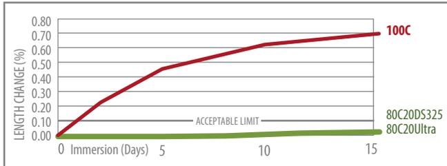
**Mortar Mix** designs tested according to a modified ASTM C1567 procedure using Type 1 cement and **Highly Reactive aggregate** in an accelerated ASR environment (80° C and 1 N NaOH solution) over 16 days.
