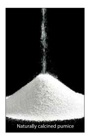
Pumice has long been recognized as the original natural pozzolan. Workability & Set Times. Pumice pozzolan-based mix designs have set times which are not significantly longer than the 100% cement control (see the University of Utah study). If a quicker set and high early strength are desired, the use of a water reducing agent will offset these properties, as needed.
